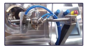
Our Schlick ABC Nano spray nozzle is pictured above. This nozzle has a spray rate of 1-10 g/min. All nozzle caps, inserts and needles are 316L stainless steel construction.
