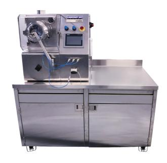
Specifically designed for our Benchtop coater, our stainless-steel workbench is pictured above. Mounted on casters with brakes, this unit can be easily relocated. Beneath the coater is plenty of space to store and conceal various coating accessories such as pans, plenums and solution preparation equipment.
