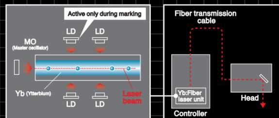
Laser beam is gradually amplified in the process of passing through fiber.
