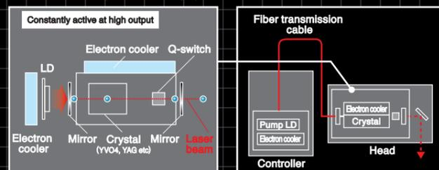
Irradiate LD (high power) light into crystal, and amplifies laser beam through round-trip reflections inside.
