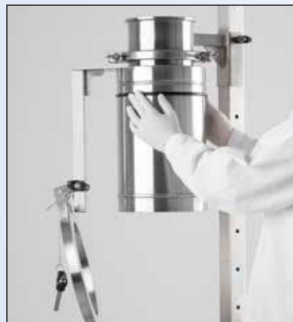
Fit the O-ring on the carrier tube
